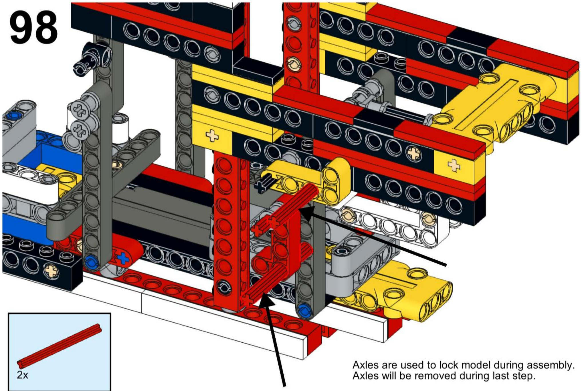
Axes are used to lock model during assembly.
